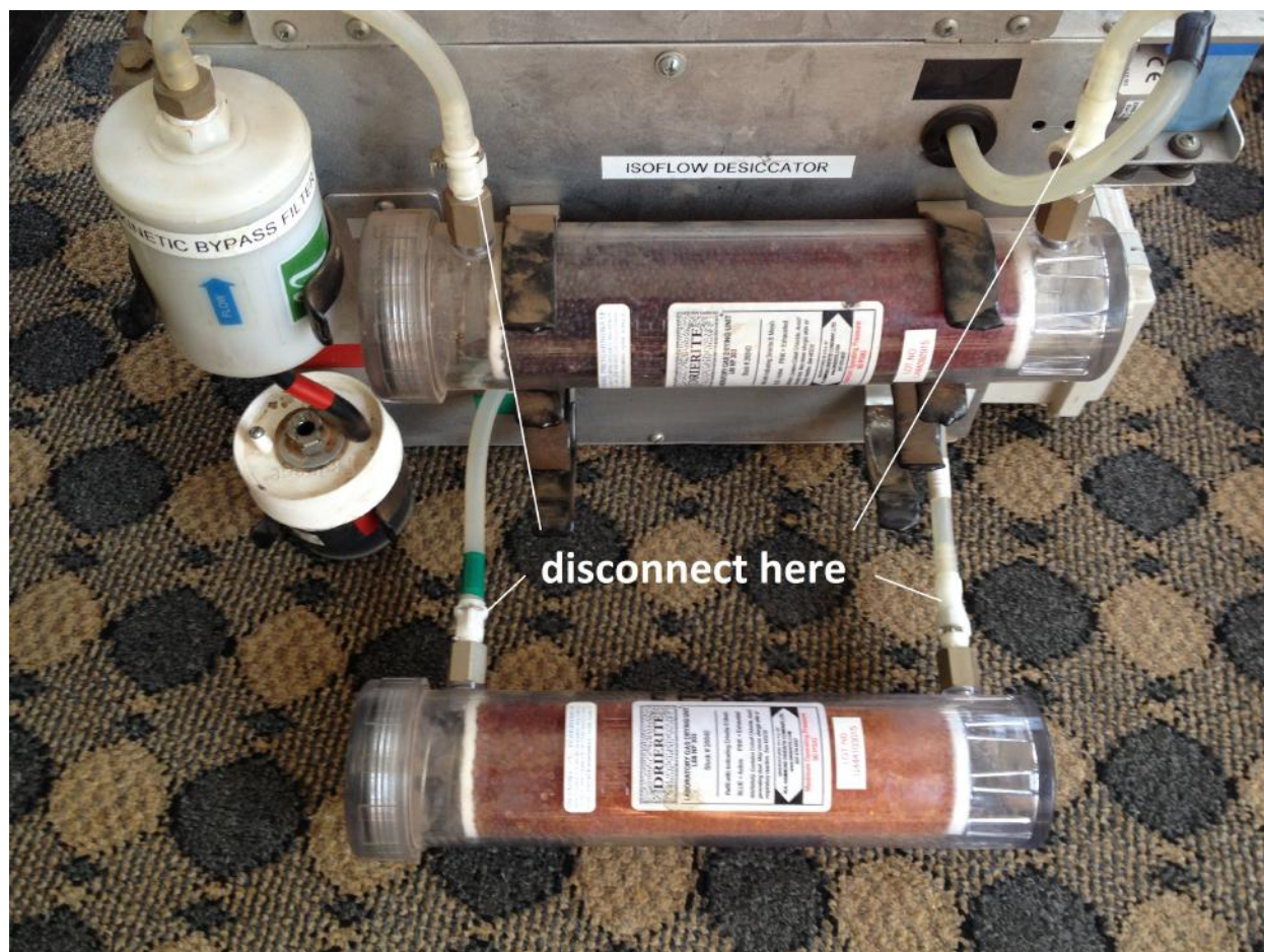
Figure 47: Removing the desiccant chamber.
