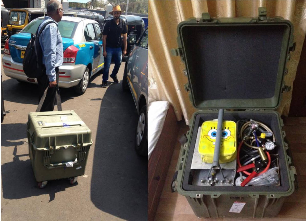
Figure 9: Sensor box case. Outside dimensions = 57 x 57 x 54 cm (L x W x H excluding wheels). The case has wheels that allow you to effortlessly roll through Customs. The wheels can be easily removed (unclipped) without hand tools. The wheels should be removed before airline travel. During sampling events, the case doubles as a work bench.
