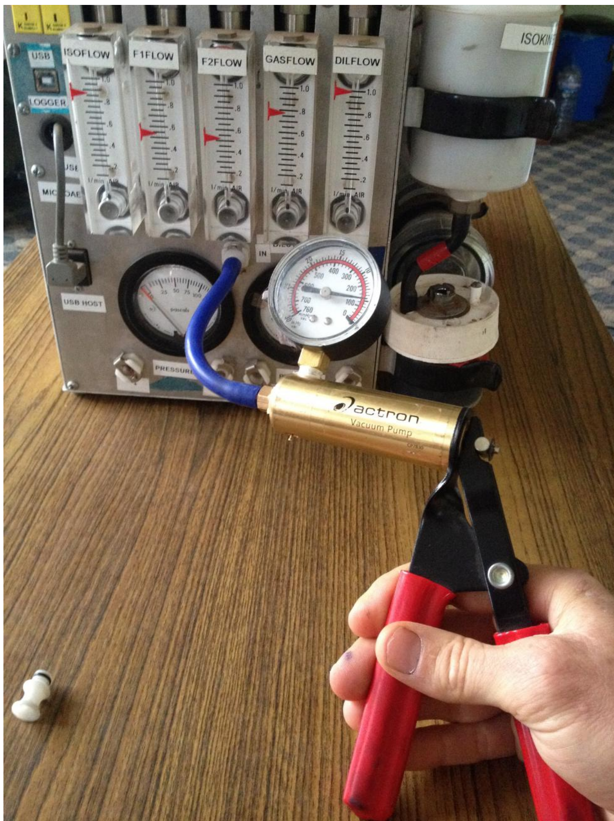
Figure 35: Leak testing the dilution train.
