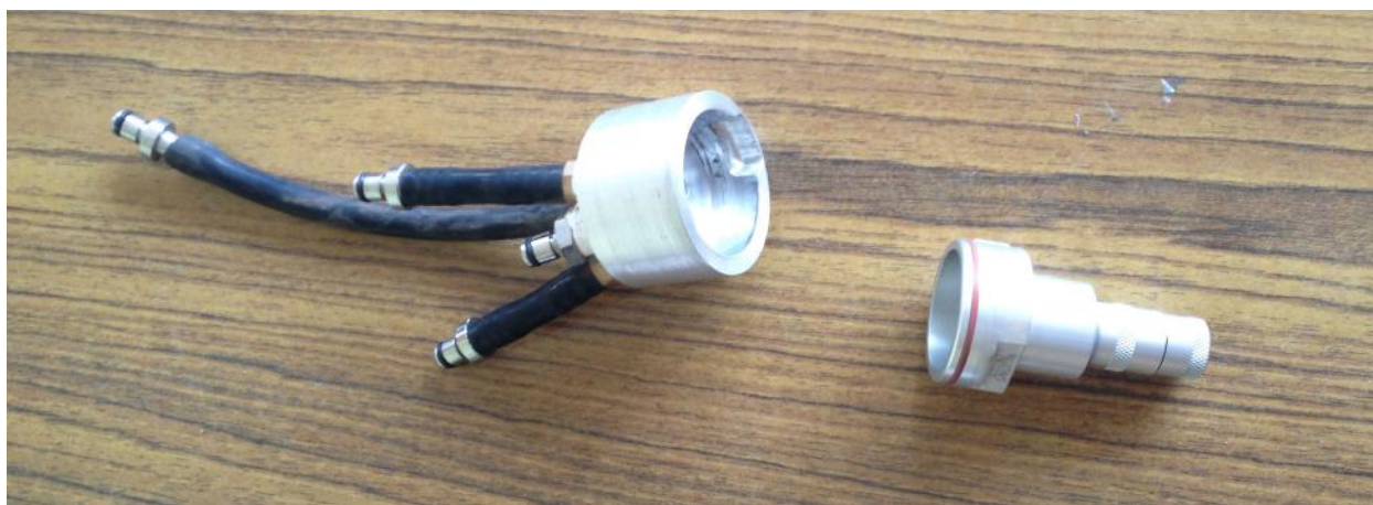
Figure 45: The cyclone outlet cap can be removed from the cyclone. Be aware of the alignment and tube connections when putting it back together.
