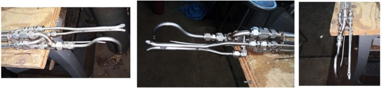
Figure 30: Probe head with nozzle and pitot tube. Positive (+) pitot port opens downward into the flow and negative (-) opens upward towards the sky. Match the + and - marks at the joints.
