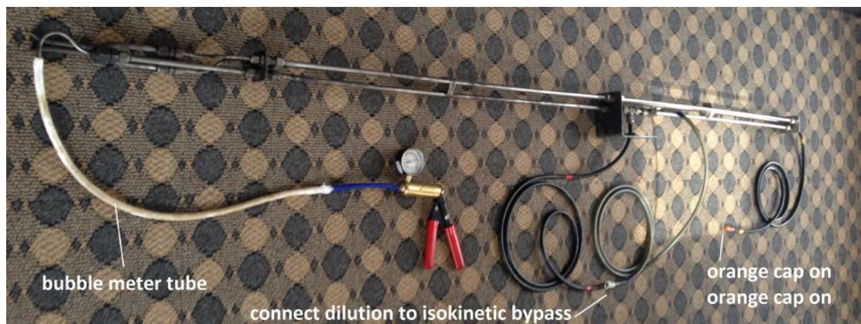
Figure 37: Leak testing the sample probe.
