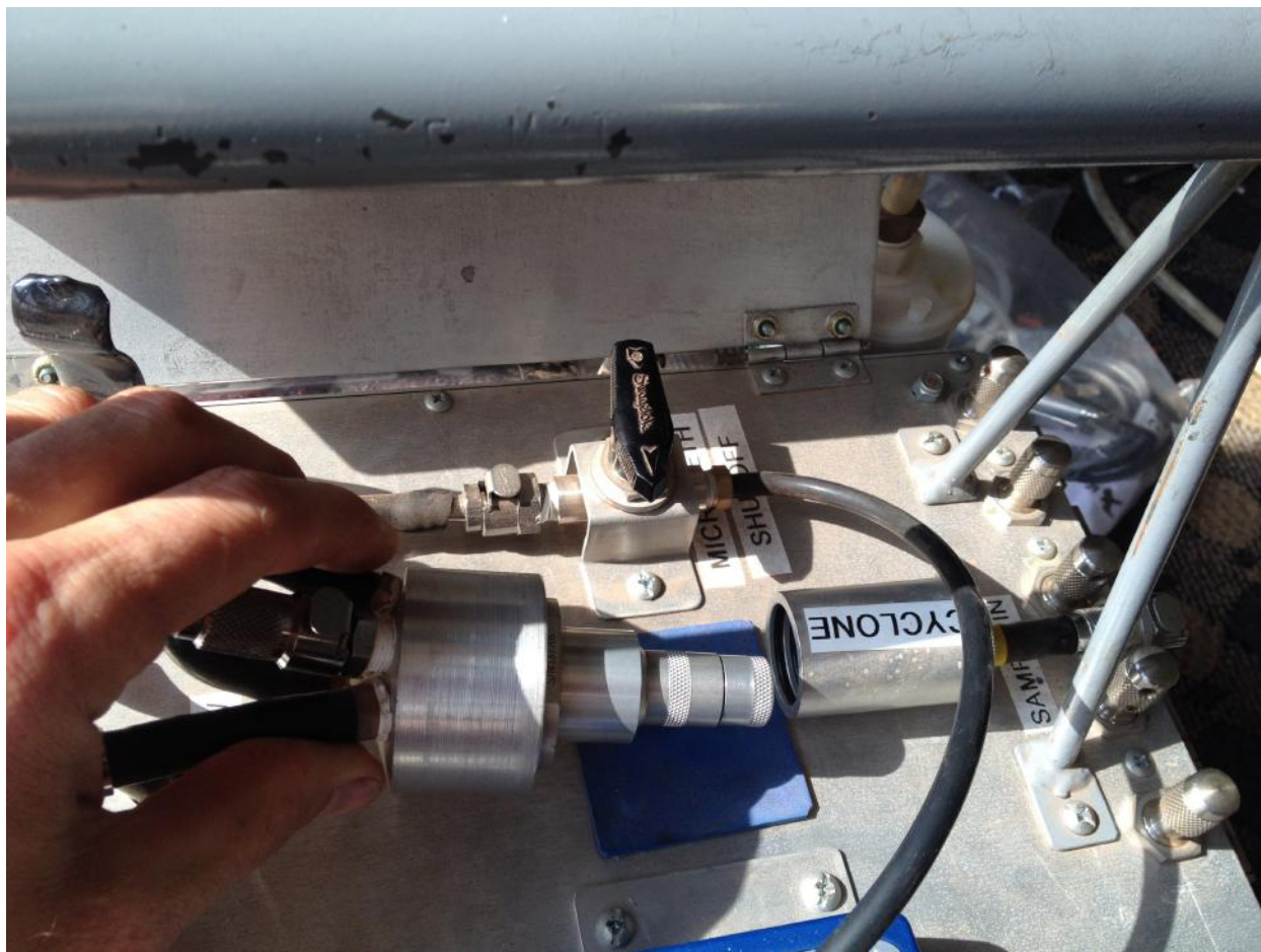
Figure 43: Slide the cyclone body apart from the inlet cap.
