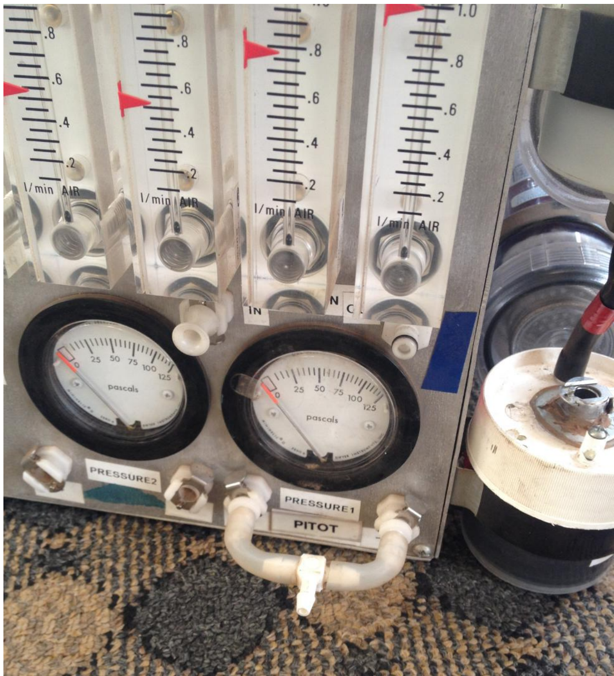
Figure 52: Connect this tube to equalize the pressure ports before zeroing.
