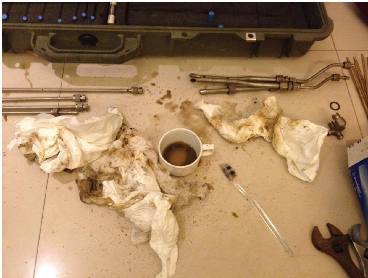
Figure 42: Cleaning the outside of the probe. You can use a tea cup from your hotel to mix the baking soda. The toothbrush will get nasty, so borrow your friend's instead of using your own.
