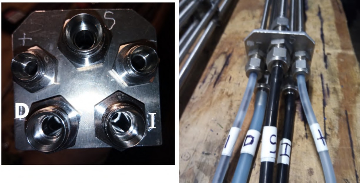
Figure 33: Connect the soft tubing to the end of the base section.
