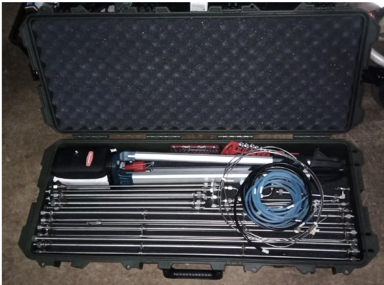
Figure 10: Probe case. Outside dimensions = 97 x 41 x 16 cm (L x W x H). The thermocouple and soft sample tubes fit inside the sensor box case.
