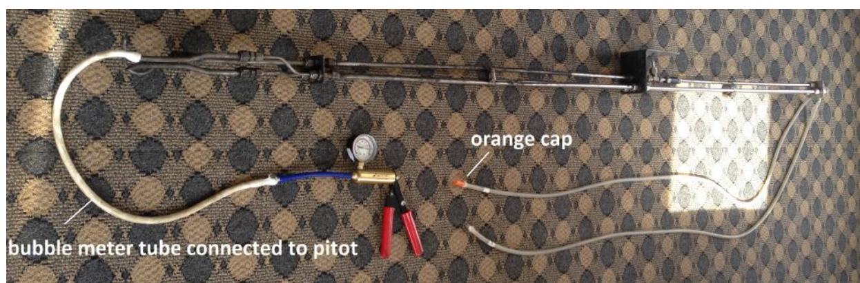
Figure 38: Leak testing the pitot tube lines.
