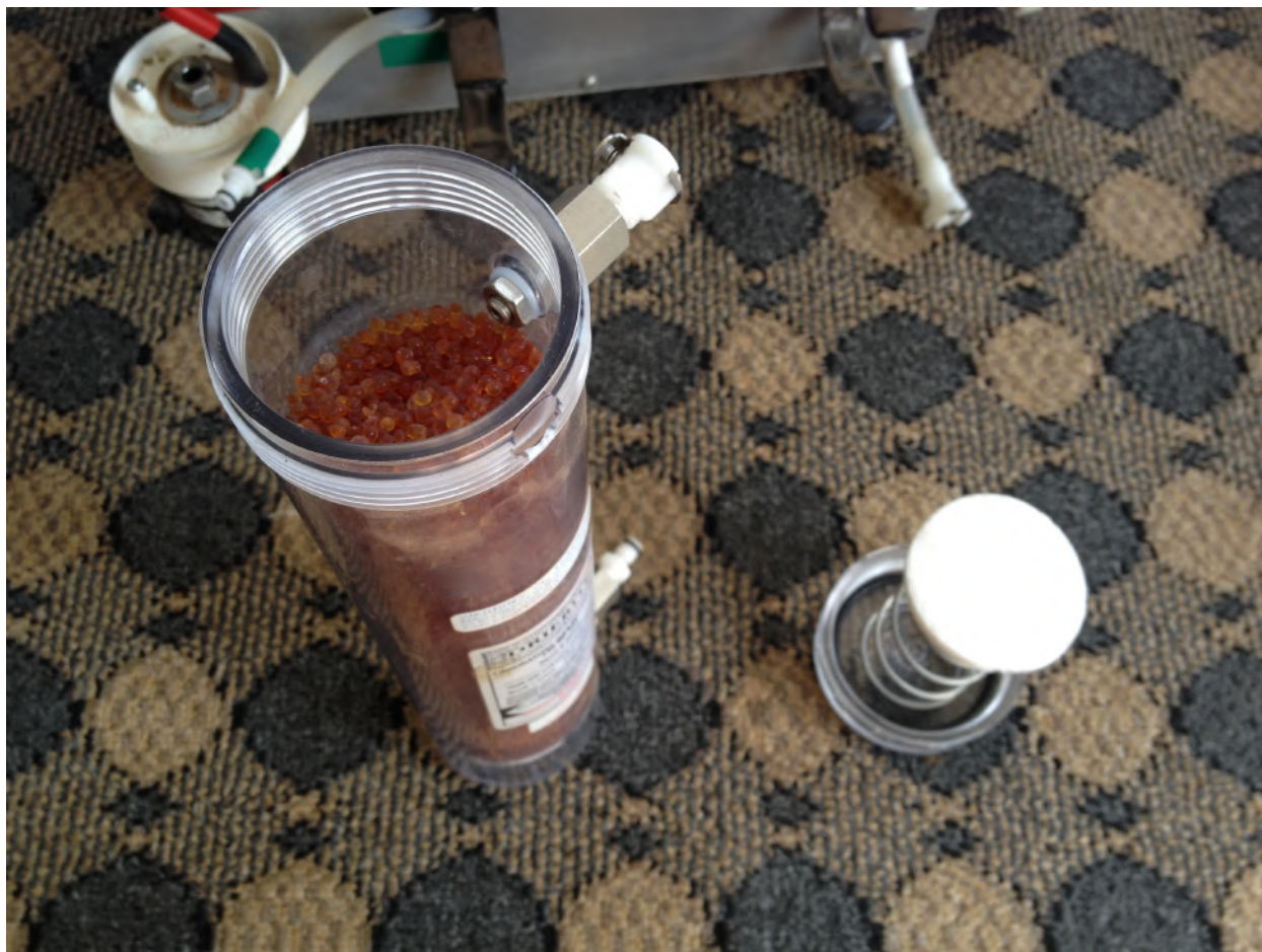
Figure 48: Removing the desiccant.
