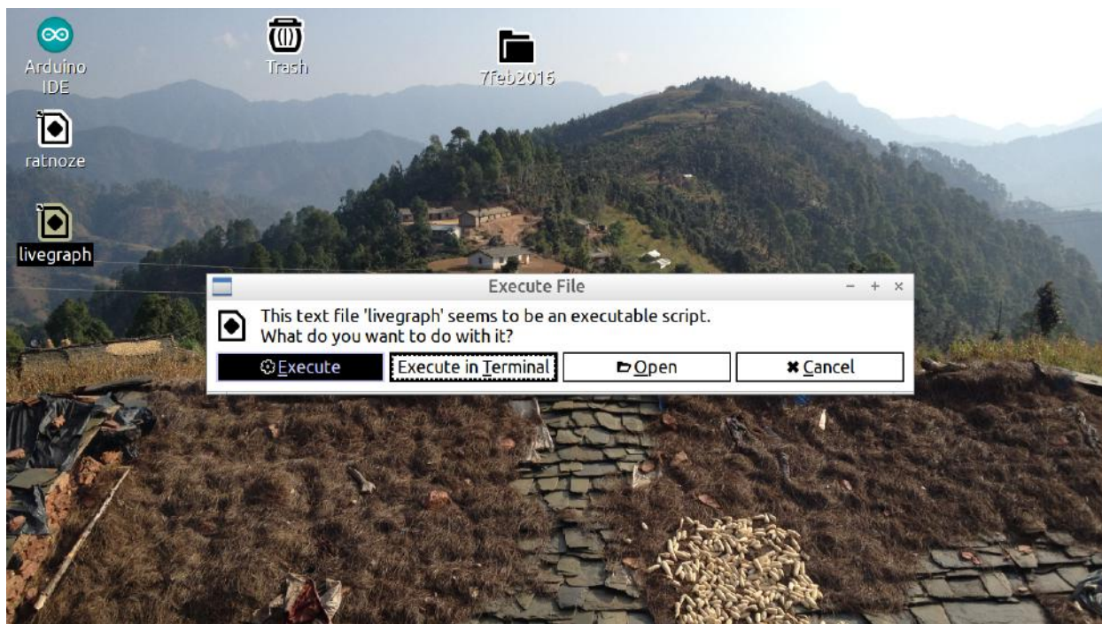
Figure 22: To launch LiveGraph, double click the livegraph desktop icon and select execute .
