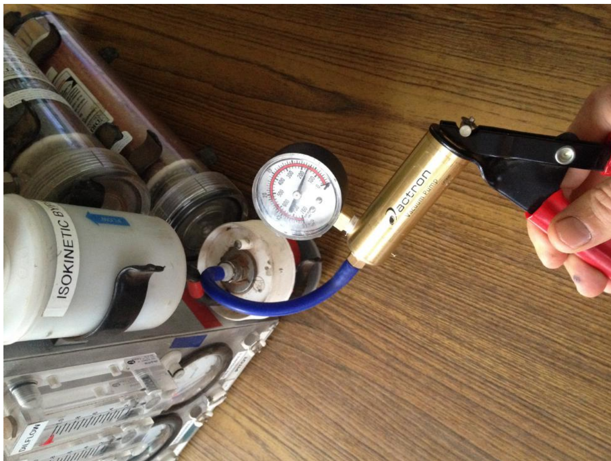
Figure 36: Leak testing the isokinetic bypass train.
