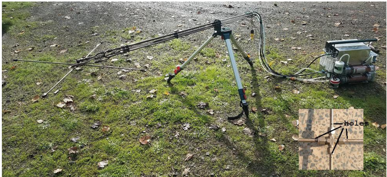
Figure 31: When assembling the multi-point array nozzle, point the holes towards the flat side of the cross (away from the elbow), so they point down when installed on the probe.
