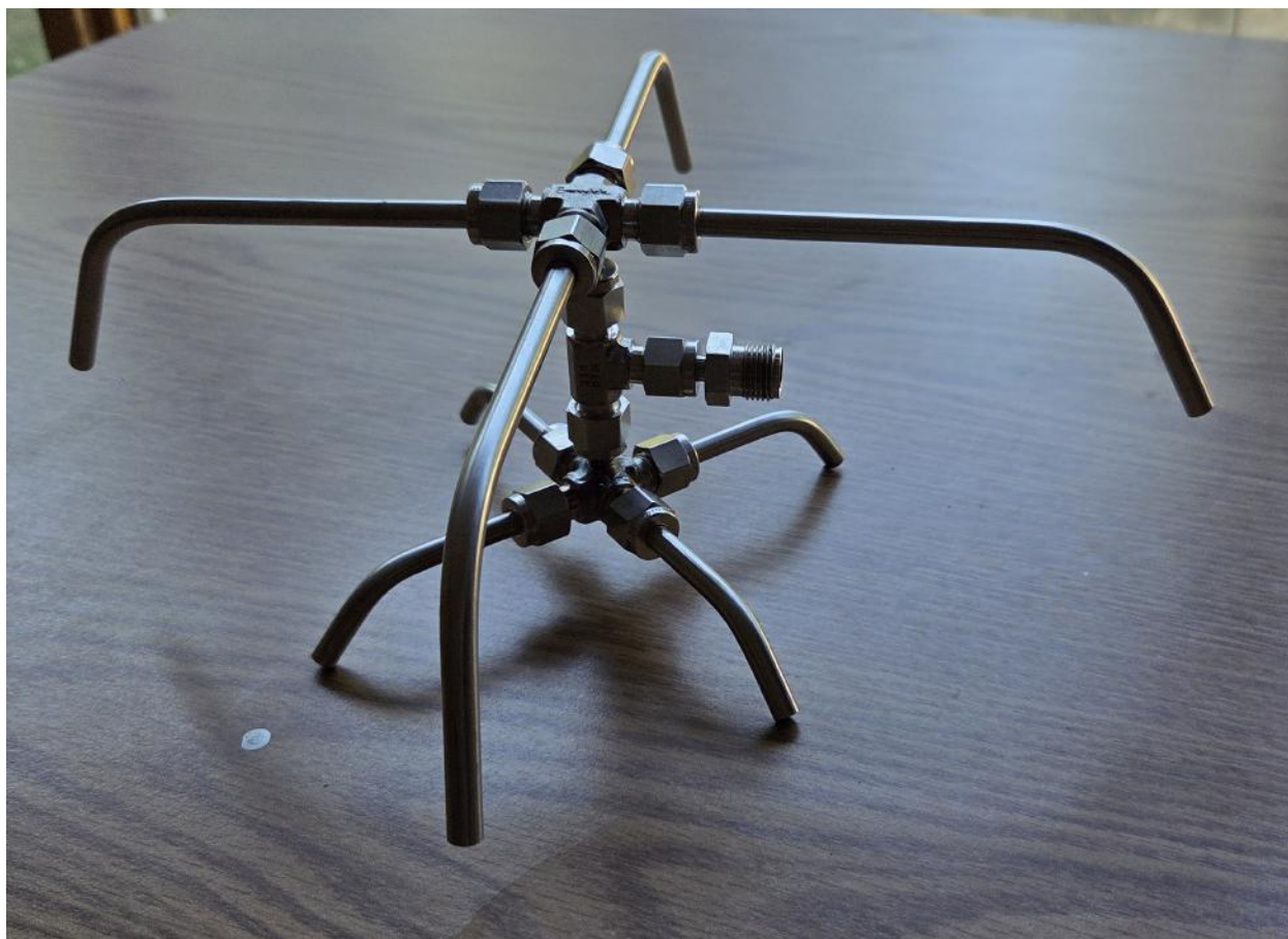
Figure 32: A multi-point nozzle for cookstoves was added in 2025 with 8 arms of 1/4" tubing, with a total diameter of 12".
