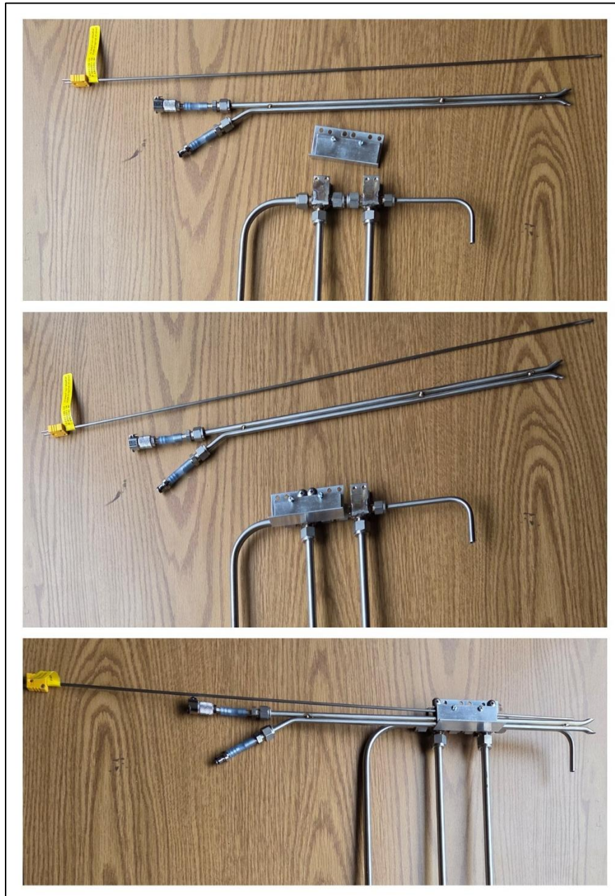
Figure 3: Pitot tube assembly including the mounting clamp, type-S pitot tube, and thermocouple. The positive pressure port has a male quick connect fitting. The negative pressure port has a female quick connect fitting.
