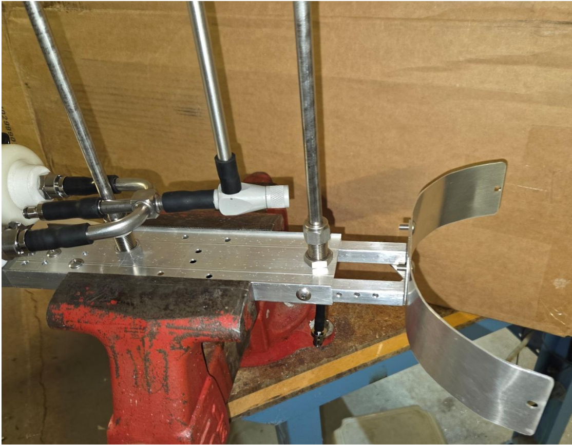
Figure 4: The chimney brace stabilizes the probe and provides an adjustable offset between the probe and the chimney to account for the size of the chimney cap. The brace can be strapped to the chimney with wire.
